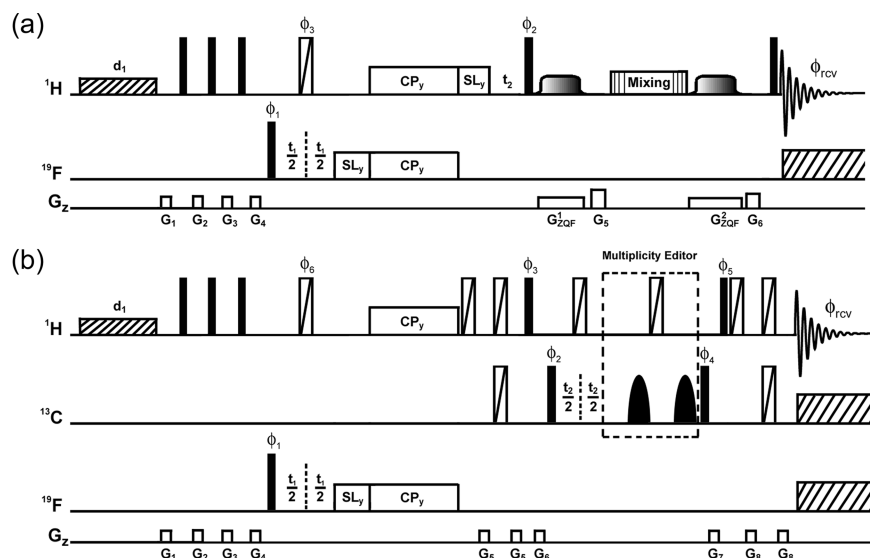
FIGURE 1. Timing diagrams of the pulse sequences used in this work. Hard 90^\circ pulses are represented by solid bars and BIPs by scored icons. Frequency-swept inversion pulses used for zero-quantum suppression are indicated by the shaded icons and adiabatic inversion pulses used in the CRISIS-type multiplicity editor (indicated by the dashed box) by solid icons. Broad-band decoupling is designated by the hatched patterns. All pulses have phase x unless noted otherwise. All gradient pulses were applied along the z -axis without shaping. All shaped pulses other than the BIPs were generated using the program Pandora's Box available as part of the Varian NMR software. Quadrature detection in the F_1 and F_2 dimensions is achieved by phase shifting \phi_1 and \phi_2 , respectively, together with \phi_{\text{rcv}} using the States-TPPI method. (a) 3D ^{19}\text{F} - ^1\text{H} heteronuclear TOCSY edited ^1\text{H} - ^1\text{H} TOCSY. The basic phase cycling is = x, -x; \phi_2 = 2(x), 2(-x); \phi_3 = 4(x), 4(-x) ; and \phi_{\text{rcv}} = x, -x, -x, x . (b) 3D ^{19}\text{F} - ^1\text{H} heteronuclear TOCSY edited, multiplicity edited ^1\text{H} - ^{13}\text{C} CRISIS-HSQC. The appropriate phase cycling is \phi_1 = x, -x; \phi_2 = 2(x), 2(-x); \phi_3 = 4(y), 4(-y); \phi_4 = 8(x), 8(-x); \phi_5 = 16(x), 16(-x); \phi_6 = 32(x), 32(-x) ; and \phi_{\text{rcv}} = \phi_1 + \phi_2 + \phi_3 + \phi_4 + \phi_5 .
